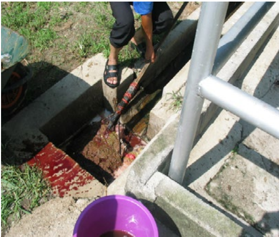
Figure 3. The abattoir wastewater flowed into the drain and solid waste was transferred into the dumping ground before being channeled into the solid trap tank.
